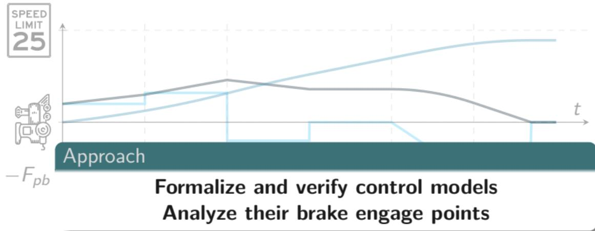
$$x' = v, \quad v' = \frac{1}{m}(-(F_g + F_r + F_c) + f_a), \quad f'_a = j \quad \& \quad -F_{pb} \leq f_a$$
