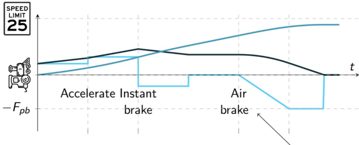
$$x' = v, \quad v' = \frac{1}{m}(- (F_g + F_r + F_c) + f_a), \quad f'_a = j \quad \& \quad -F_{pb} \leq f_a$$
